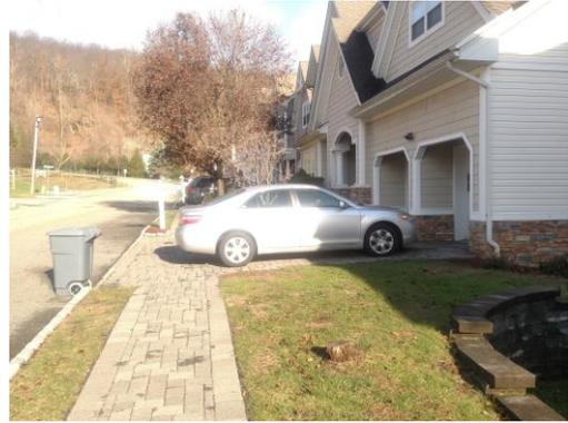
**The 22 ft. offset model does not allow sufficient length for parking. Note the trash cans in street due to lack of space.**
